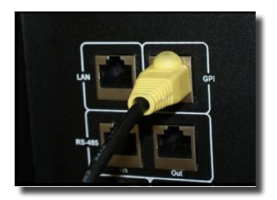
4. With the monitor OFF plug the provided update cable (RJ-45 to USB) into the monitor's GPI Port.
