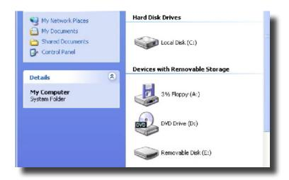
7. Plug the update cable (RJ-45 to USB) into a USB Port on your computer. It may take a few moments for the computer to recognize your monitor as a USB Mass Storage Device so please be patient. Once recognized the monitor will appear in the explorer window as an attached drive.
