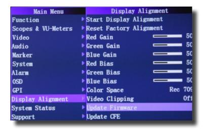
9. After the computer has finished copying the entire firmware file to the monitor's memory go the monitor's Display Alignment Menu and select the Update Firmware Option.
