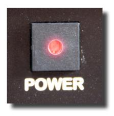
3. Next turn the monitor off from the keypad by pressing the power button, but keep the monitor plugged in.
