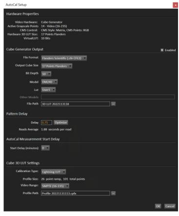
Verify your CR100 probe is centered in front of the screen and select OK from the AutoCal Setup window in Calman to begin the profiling process. Once the profile is complete your LUT file will be stored in the location previously selected.
