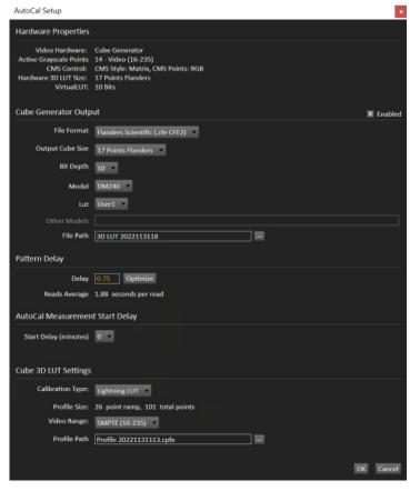
Verify your i1 probe is centered in front of the screen and select OK from the AutoCal Setup window in Calman to begin the profiling process. Once the profile is complete your LUT file will be stored in the location previously selected.
