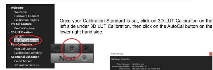
In the AutoCal Setup Window set the File Format to FlandersScientific (.cfe CFE2) and then select your monitor model from the drop-down list.
