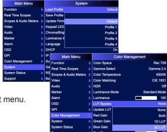
Bypass the 3D LUT in the monitor's Color Management menu. Color Management > LUT Bypass > 3D LUT.
