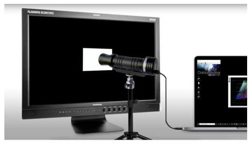
Plug the CR100 into the computer and aim it towards the middle of the monitor.
