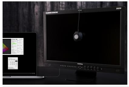
Connect the i1D3 probe to the computer and place it in the middle of the monitor with the diffuser open.
