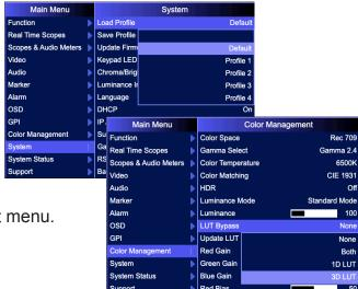
Bypass the 3D LUT in the monitor's Color Management menu. Color Management > LUT Bypass > 3D LUT.
